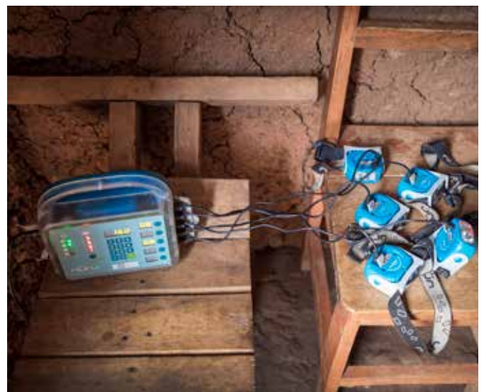
Up to five headlights can be charged at once with the 'Octopus' Photo: Sven Torfinn/ENERGIA
