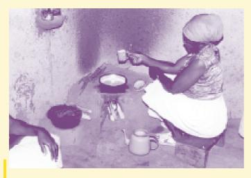
The UPESI (or Maendeleo) stove, which was developed in Kenya, is based on a standard ceramic liner that can be produced and used by artisans and women in the informal sector. The stove uses about 40% less fuel than three-stone open fires, producing up to 60% less smoke. (Photo: Courtesy of ITDG-Kenya)
