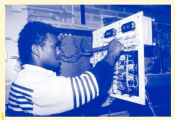
Nixon Silas Pio testing a microhydro distribution box in the APACE/UTS Renewable Energy Laboratory (Photo: Donnella Bryce)
