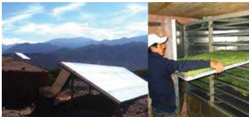
Source and Photo: Two unit rack solar dryer (left) and cabinet dryer (right), C. Mueller, Fundación EcoAndina
