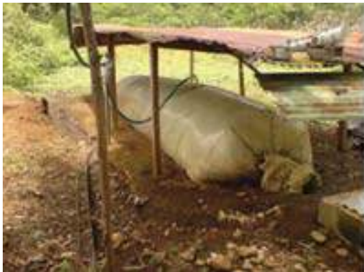
Source and photo: Biodigester “Taiwan” model, Earth University’s Community Development Programme, F. Schmitt
